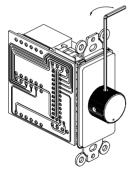
Figure 1 Removing the Knob
